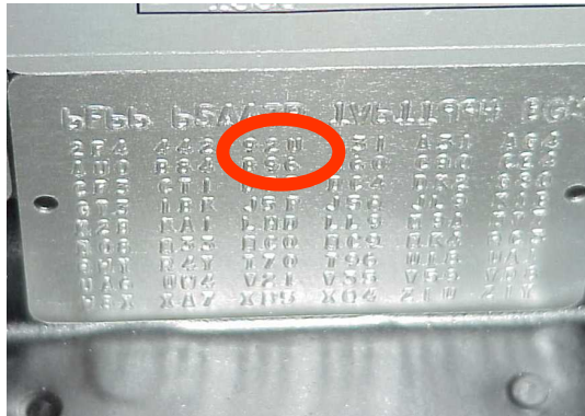
VIN PLATE FRONTERA PAINTCODE = 92U
